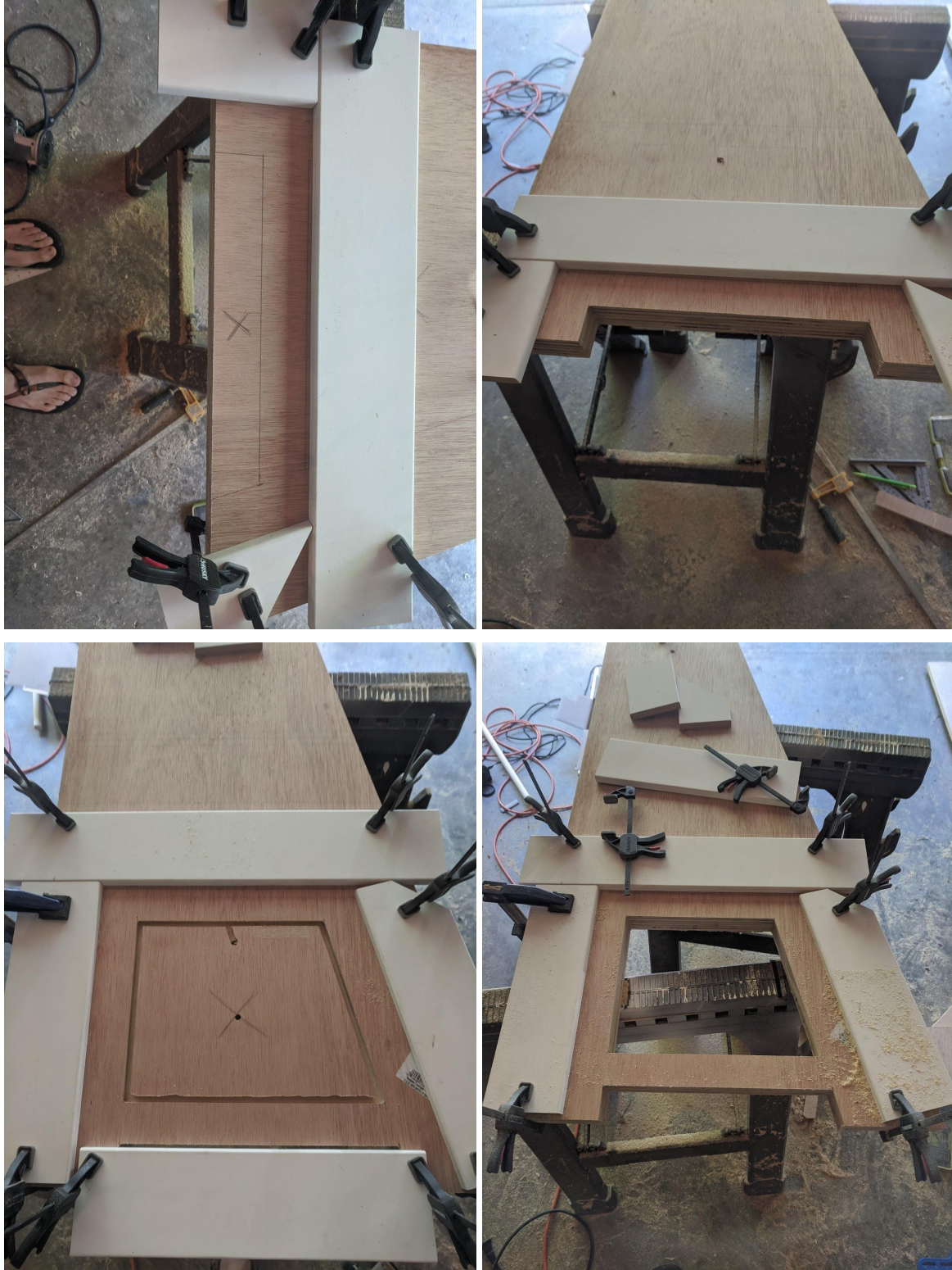
Figure 8: set up your router fences and cut into both boards at once via many passes of a cutting bit. Note that the fences should be offset by the distance from your bit edge to the edge of the flat router floor.
