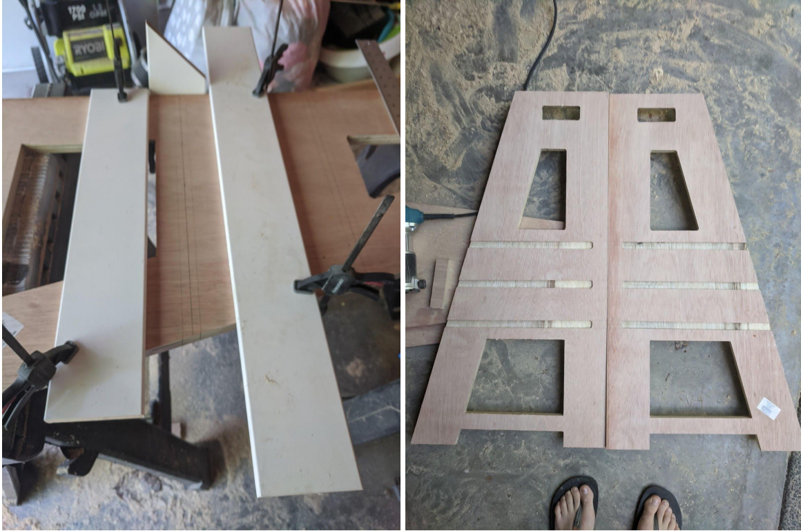
Figure(s) 12: set up your fences again (note the fence at the top stops the router from cutting past that 1.5" setback) and get routing! (Halfway through your plywood or less). Note: you can also do this with a "poor man's router" - a combo of wood and a chisel. YouTube it.
