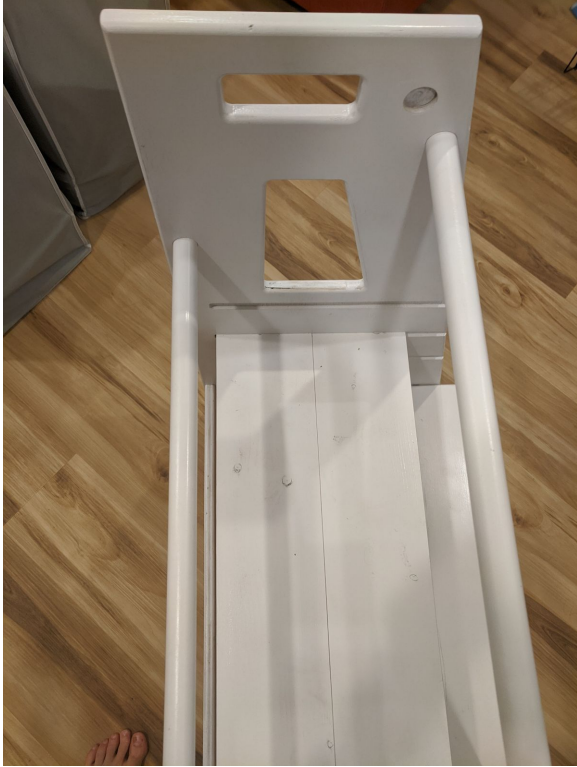
Figure 14: an overhead view of the finished helper, to illustrate where 1" circular recesses should be drilled to facilitate dowel rod installation.
