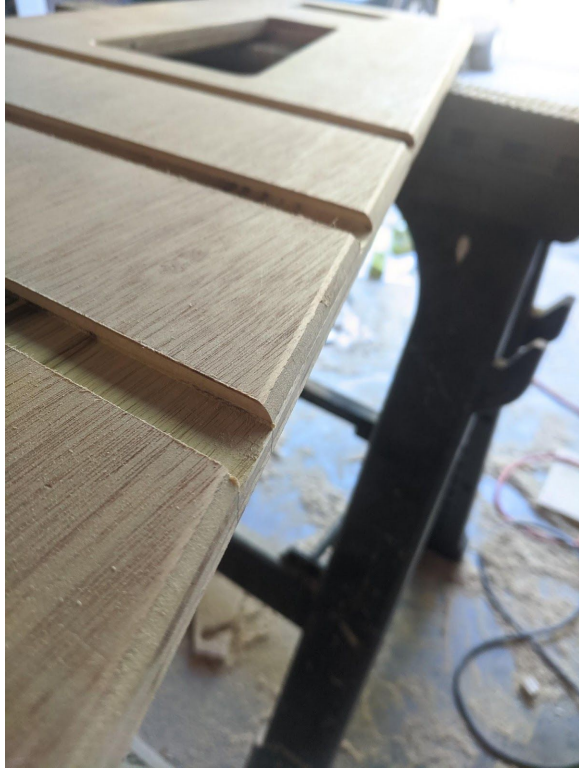
Figure 13: round over bits make this super easy. I can't believe it took me this long to buy a router.
