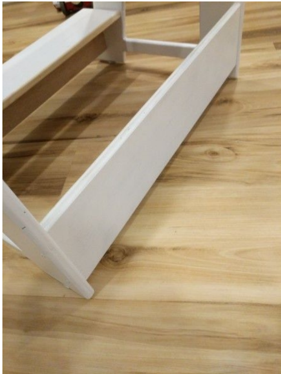
Figure 15: a view of the bottom support board. This board is screwed in to secure the bottom of the vertical (counter-facing) edge of the Helper.
