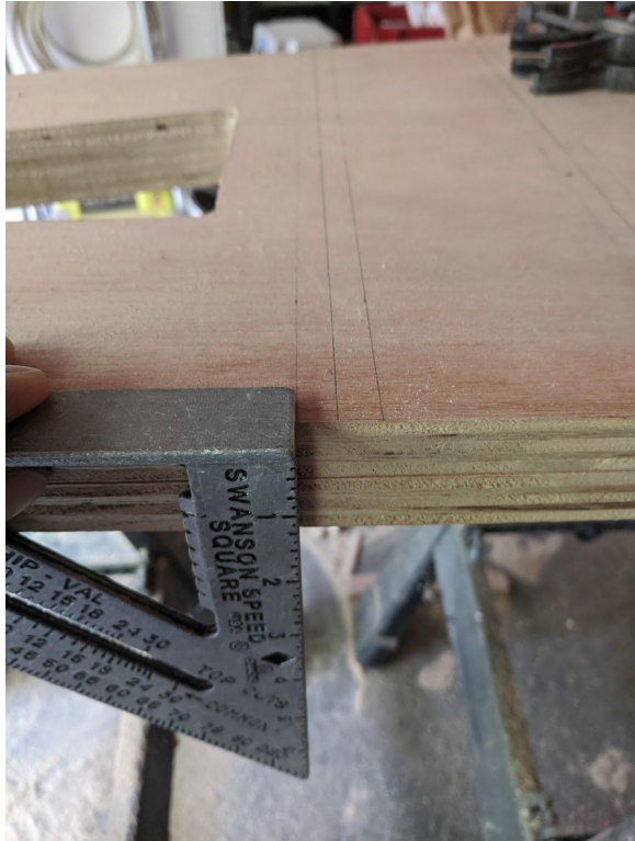
Figure 9: We're looking directly at the 20" guide line now, and the lines around it that denote the bounds of the \frac{3}{4} plywood. On the far right side, you'll see the 18" lines.
