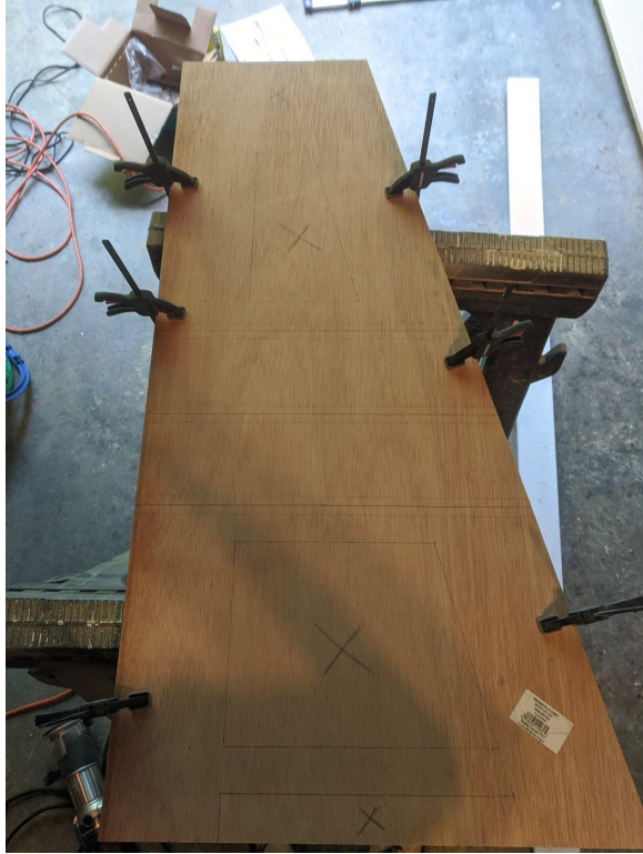
Figure 6: here's a picture of my cutouts drawn on the plywood. Note the parallel, horizontal lines in the middle of the board. That's where the platform will get bolted in (three options). So don't let your cutouts get too close to that zone!
