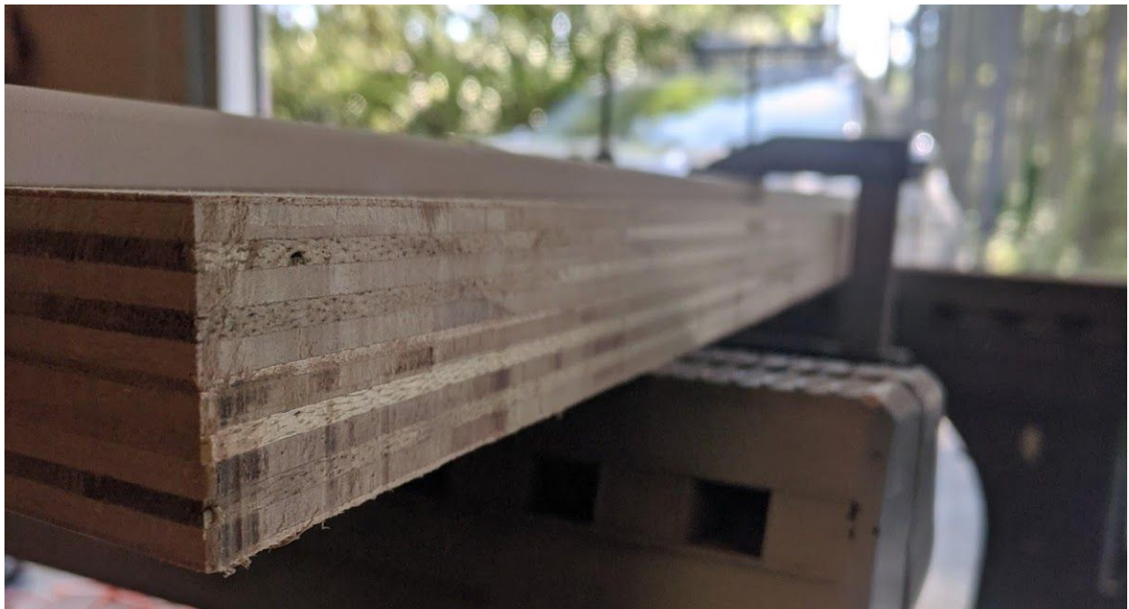
Figure 4: That's two pieces of plywood stacked on top of one another. You'll keep them clamped together this way for nearly the entire build.
