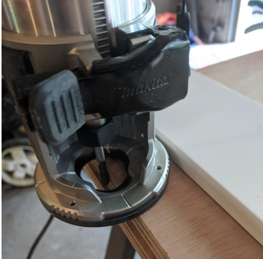
Figure 3: The router rides along the fence, making multiple passes through both boards to make them identical.
